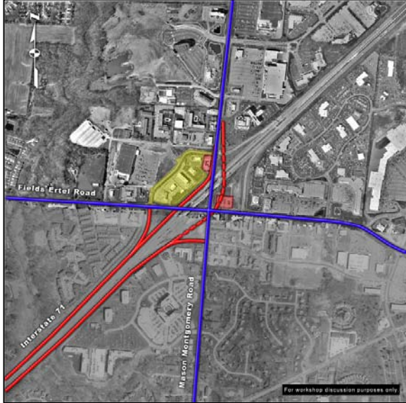
Figure 23 – Directional Ramp Improvement to the Fields Ertel/Mason Montgomery Interchange with I-71
